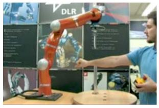
They fitted an articulated robotic arm with various tools (scalpel, kitchen knife, scissors, steak knife, and screwdriver) and programmed it to execute different striking maneuvers. They used a block of silicone, a pig's leg, and at one point a human volunteer's bare arm as their, uh, test surface.
